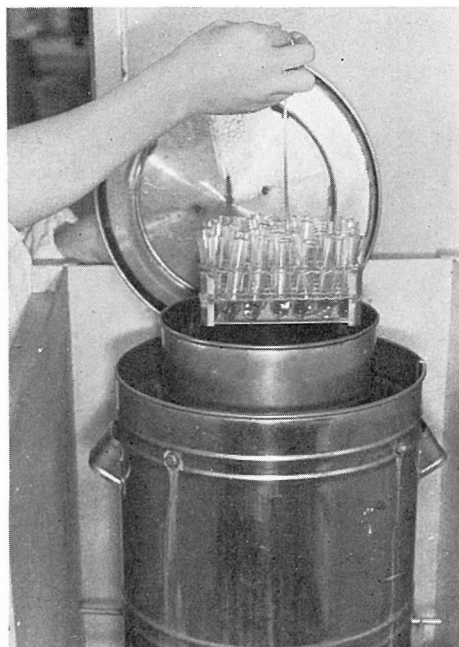
Photo 1. Double-Walled Heating Bath (Shows wire basket with test tubes being introduced to it.)
