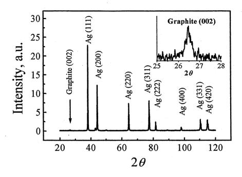
Fig. 4. XRD pattern of Ag/graphite coating deposited at 3 cm distance from the nozzle exit. The zoom part of the figure shows the characteristic peak  $(2\theta = 26.4 \text{ degree})$  of graphite (Graphite-2H, hexagonal)
