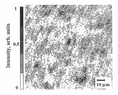
Fig. 3 EPMA characteristic X-ray images of C inclusions into the Ag matrix presented as a gray scale.
