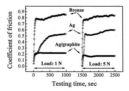
Fig. 5. Frictional characteristics of the Ag and Ag/graphite coatings prepared at 3 cm distance from the exit nozzle and bronze. In this case substrates were fixed.
