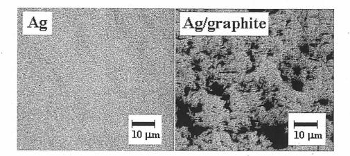
Fig. 2 OM cross-sectional view of the Ag and Ag/graphite overlays.
