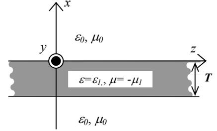
**Fig.2** Finite-thickness slab with negative permeability.
