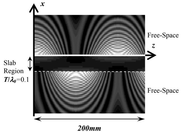
Fig.5 The field distribution,  $|H_z|$ , along the slab with negative permeability material for the thickness  $T/\lambda_0=0.1$ . The other parameters are the same as those in Fig.3.
