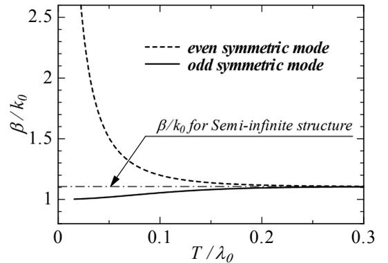
**Fig.3** The normalized propagation constant as a function of normalized slab thickness, where  $\varepsilon / \varepsilon_0=1.144$  and  $\mu / \mu_0=-6.071$ , respectively, at the fixed operating frequency 13.6GHz.
