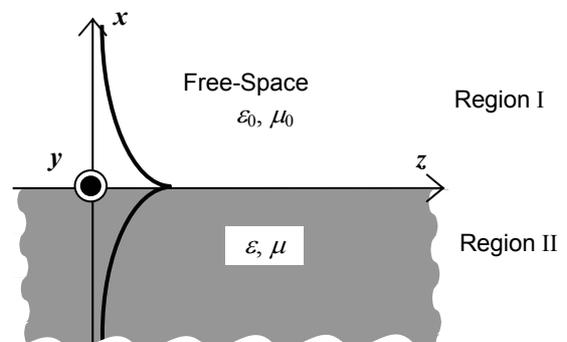
**Fig.1** Semi-infinite single negative material and surface wave along it.
