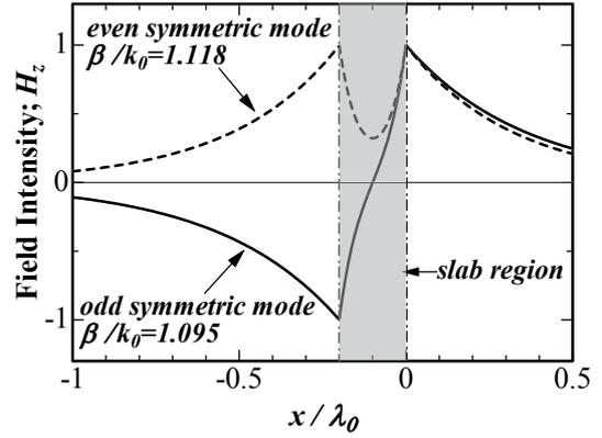
Fig.4 The mode profiles of the longitudinal field component,  $H_z$ , for each surface-wave at the normalized slab thickness  $T/\lambda_0=0.2$ . The other parameters are the same as those in Fig.3.
