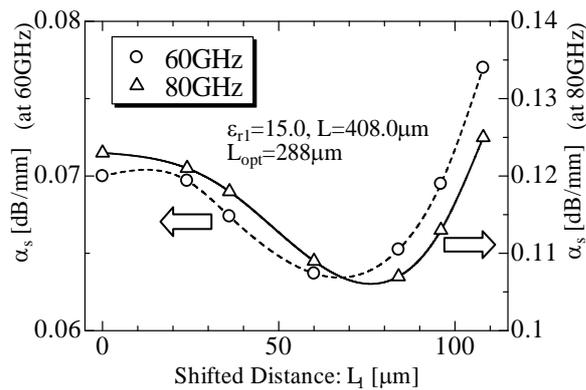
**Fig.5** Leakage loss characteristics for the AGS dielectric sheets location at operating frequency is 60GHz and 80GHz.
