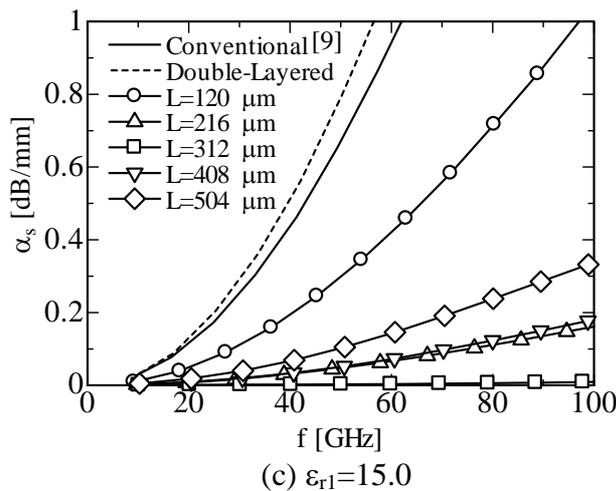
**Fig.2** Leakage loss characteristics for AGS dielectric sheets backing CBCPWs as a function of the operating frequency where  $h_1=40.0\mu\text{m}$  and the air-gap width is a parameter.
