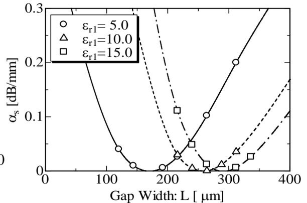
**Fig.3** Leakage loss characteristics for CBCPW with AGS dielectric sheets as a function of air-gap width at  $80\text{GHz}$  where the permittivity of the dielectric sheet is a parameter.
