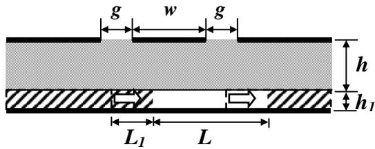
**Fig.4** Tolerance of AGS dielectric sheets position. The  $L=408.0\mu\text{m}$  width air-gap between the dielectric sheets is shifted  $L_1$  toward the right.
