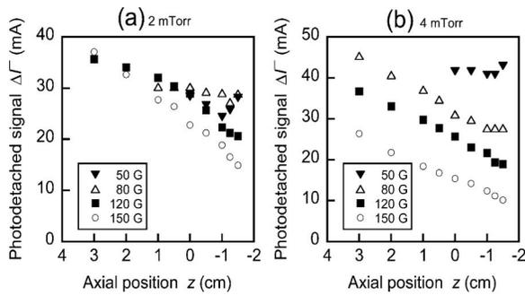
FIG. 4. Axial distributions of negative ion production in H<sub>2</sub> plasmas for two different gas pressures: (a)  $p(\text{H}_2)=2$  mTorr and (b) 4 mTorr. Parameter is the intensity of the MF,  $B_{\text{MF}}$ .
