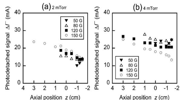
FIG. 3. Axial distributions of negative ion production in  $D_2$  plasmas for two different gas pressures: (a)  $p(D_2)=2$  mTorr and (b) 4 mTorr. Parameter is the intensity of the MF,  $B_{MF}$ .
