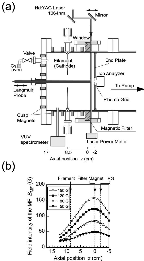
FIG. 1. (a) Schematic diagram of the ion source. The probe, the laser path, and power meter used in photodetachment experiments are also shown. (b) Axial distributions of field intensities for four different MFs.
