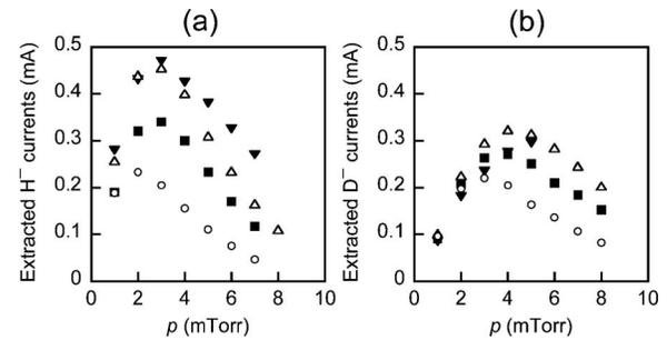
FIG. 6. Pressure dependence of extracted (a) H<sup>-</sup> and (b) D<sup>-</sup> currents, corresponding to the negative ion densities shown in Fig. 5, where extraction voltage  $V_{\text{ex}}=1.5$  kV.
