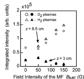
FIG. 7. The integrated intensities of VUV spectra for two different positions as a function of  $B_{\text{MF}}$ . Experimental conditions are as follows:  $V_d=70$  V and  $I_d=10$  A.
