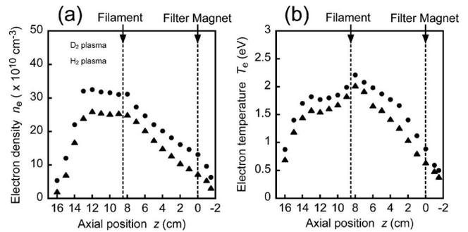
FIG. 2. Axial distributions of plasma parameters (a)  $n_e$  and (b)  $T_e$  in  $H_2$  and  $D_2$  plasmas. Experimental conditions are as follows:  $V_d=70$  V,  $I_d=5$  A, and  $p(H_2)=p(D_2)=1.5$  mTorr.
