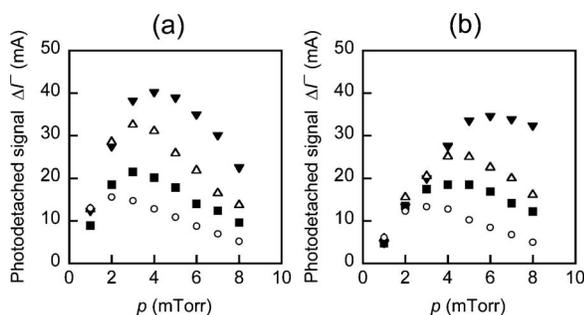
FIG. 5. Pressure dependence of negative ion densities in the vicinity of the extraction electrode: (a) H<sup>-</sup> density and (b) D<sup>-</sup> density. Parameter is the magnetic field intensity  $B_{\text{MF}}$  of the MF,  $B_{\text{MF}}=50\text{G}$ ( $\blacktriangledown$ ),  $80\text{G}$ ( $\triangle$ ),  $120\text{G}$ ( $\blacksquare$ ), and  $150\text{G}$ ( $\circ$ ). Experimental conditions are as follows: discharge voltage  $V_d=70$  V and discharge current  $I_d=10$  A.
