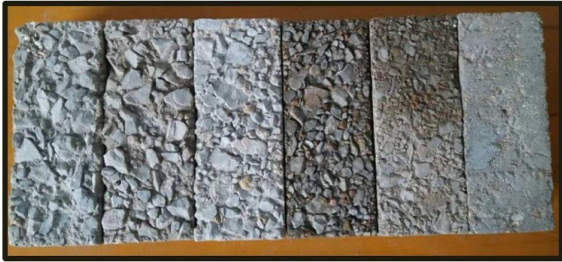
Figure 3.3. concrete surfaces with different roughness [9]
