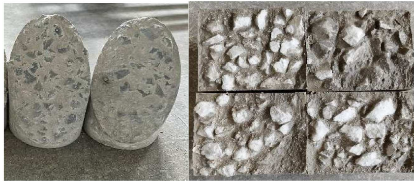
Figure 3.4. Surface roughness preparation in this research
