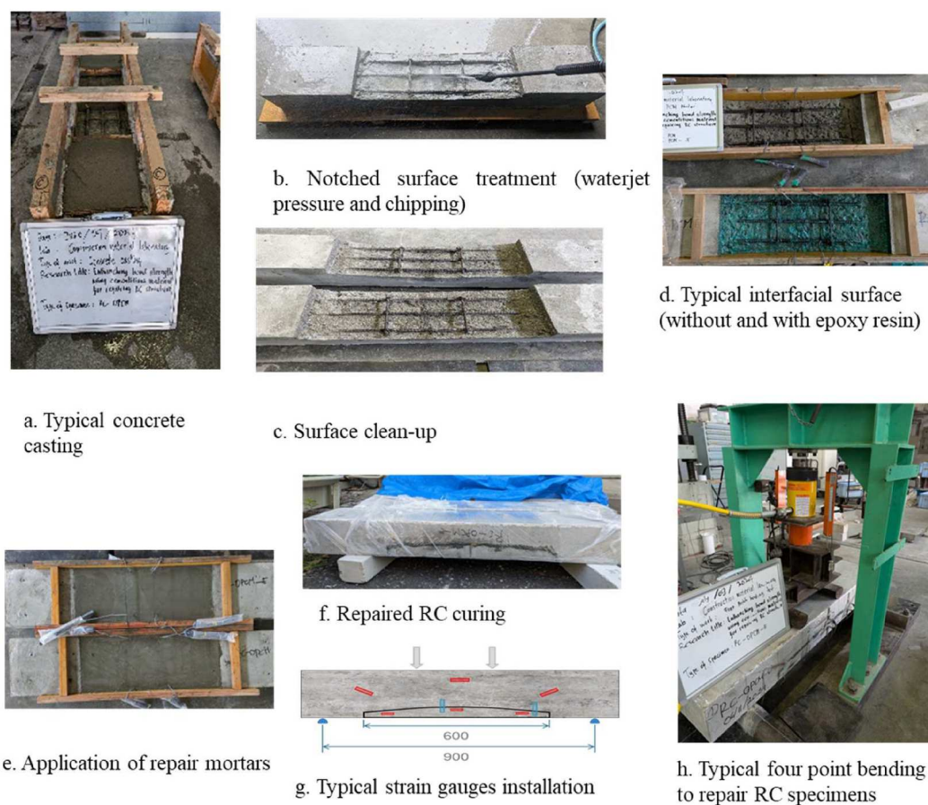
Figure 6.6. Typical repaired RC specimen preparation and testing
