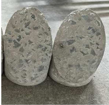
Figure 4.5. Surface roughness preparation for the slant shear test
