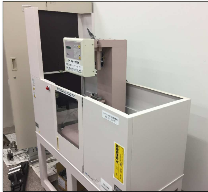
Figure 3.6: Izod-Charpy impact test machine (CIT-25JCI) for evaluating the impact resistance of test specimens.
