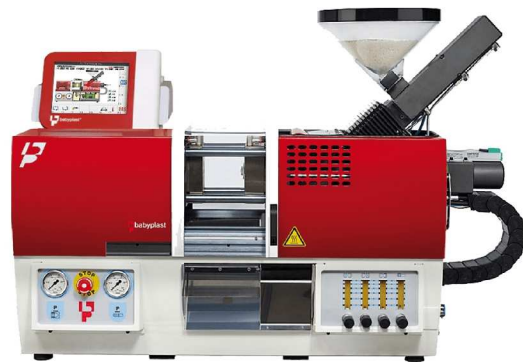
(c) Injection molding machine (Babyplast 6/10P, Rambaldi + Co. I.T. Srl).
