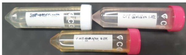
Figure 3.1: Acrylic paint coating agent (SHP470-FT2050, Momentive Co., Ltd.) with varying CNF content: 0 wt%, 1 wt%, and 4 wt%.
