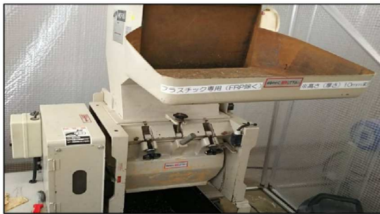
(b) Pulverizing machine (U-280, ZI-420 type, Horai Co., Ltd.).
