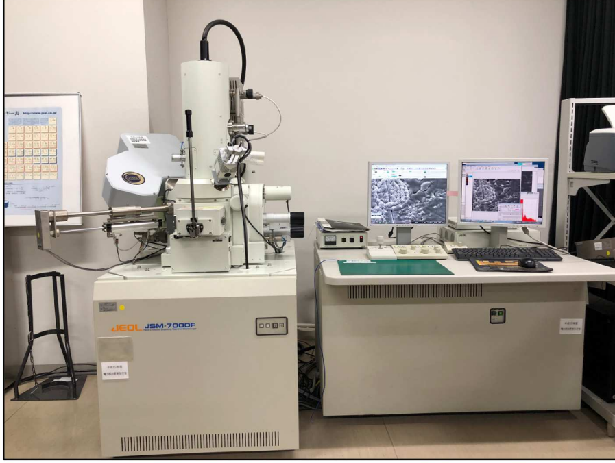
Figure 2.10: Field emission scanning electron microscope (FE-SEM; JSM-7000F, Japan Electron Optics Laboratory Co., Ltd., Akishima, Tokyo, Japan) used for surface and fracture morphology analysis of composite specimens.
