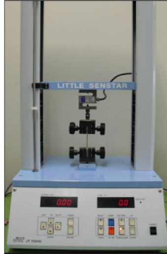
Figure 2.11: Universal testing machine (LSC-1/30D, JT Tosi, Japan) used for evaluating the tensile properties of molded specimens and laminating films.
