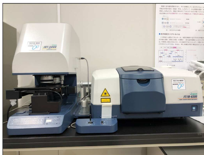
Figure 2.8: Fourier Transform Infrared Spectrometer (FT/IR-6300, JASCO, Tokyo, Japan) used for spectral analysis of PP and PET films.
