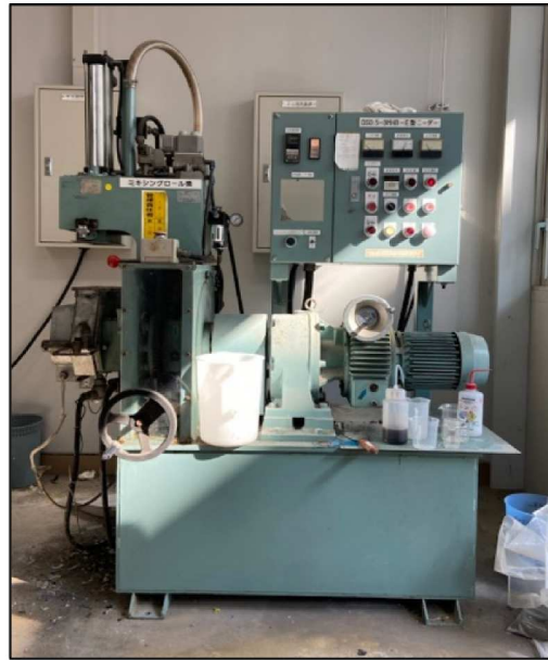
(a) Kneader (DS0.5-3MHB-E, Satake Chemical Machinery Industry Co., Ltd.).
