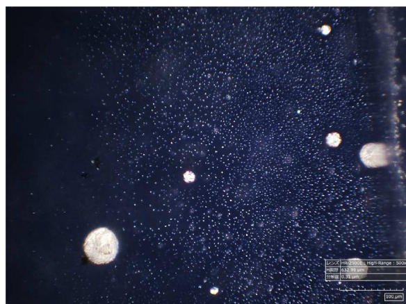
Figure 4-4-2-1. Image of 5wt% [BMIM][TFSA] gel formed by compound 1-8 observed by a digital POM ( \times 500 ).
