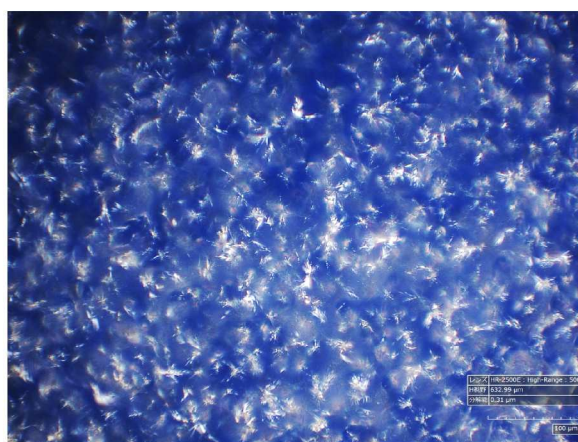
Figure 4-4-2-3. Image of 5wt% [BMIM][TFSA] gel formed by compound 2-F observed by a digital POM ( \times 500 ).
