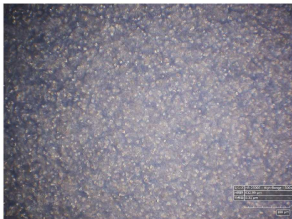
Figure 4-4-2-4. Image of 5wt% [BMIM][TFSA] gel formed by compound 3-8 observed by a digital POM ( \times 500 ).
