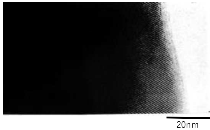
Fig. 2-1-9 TEM image of Si 3 N 4 powder synthesized by silicon metal nitridation method.
