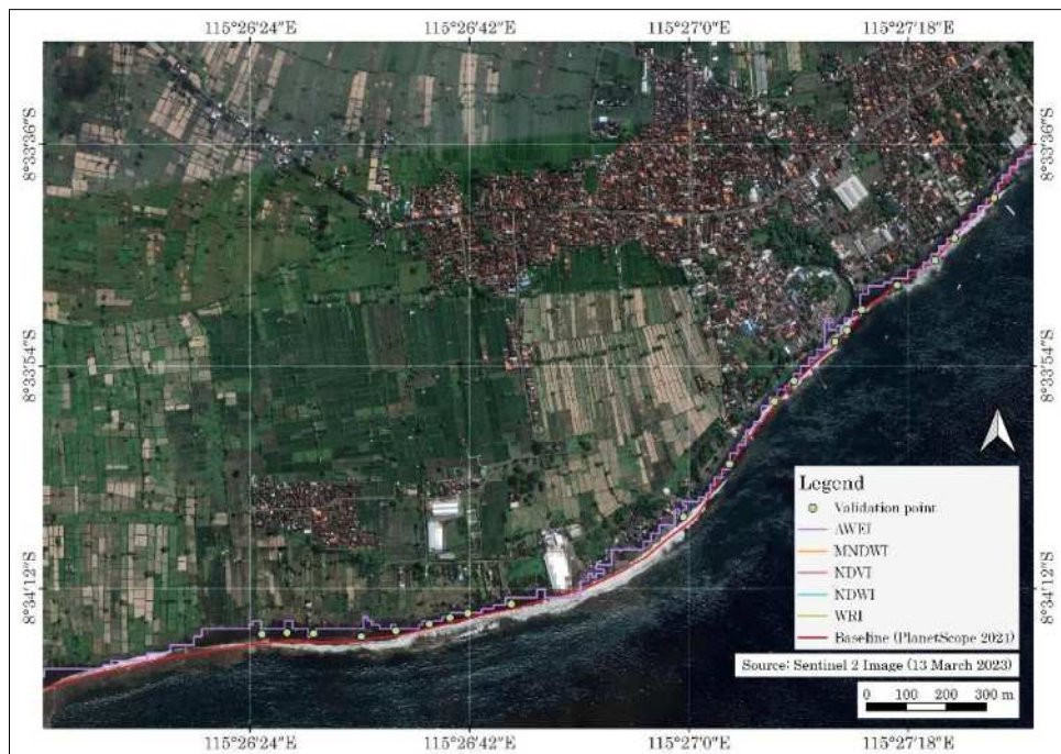
Figure 6-10. Result of coastline extraction using Automated Water Extraction Index (AWEI).
