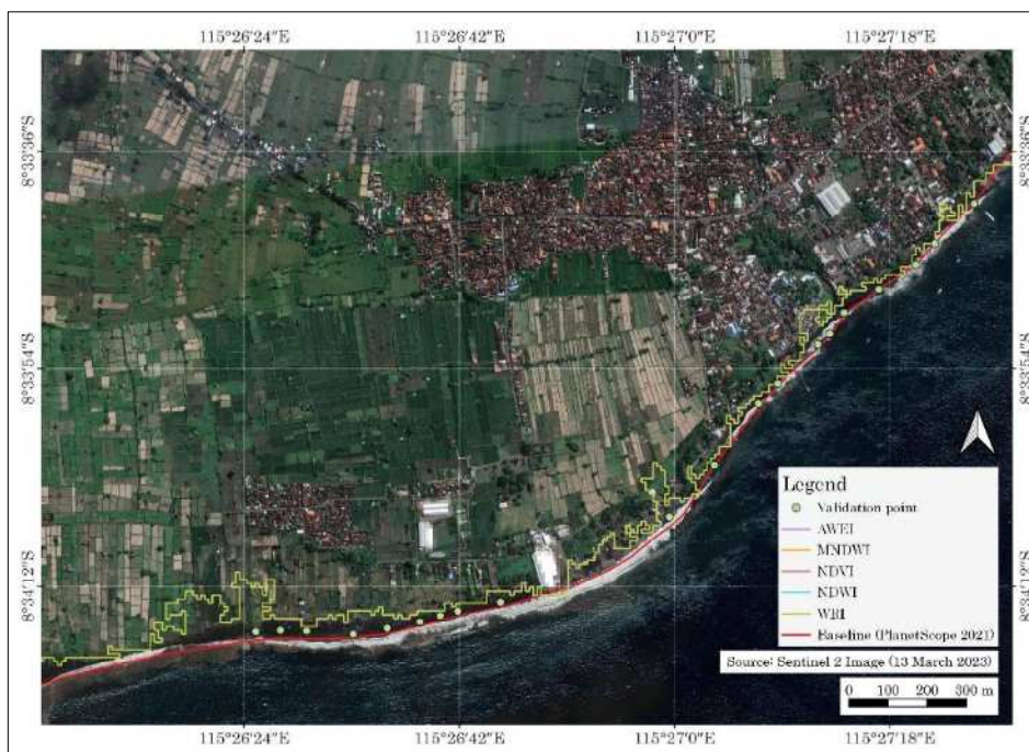
Figure 6-9. Result of coastline extraction using Water Ratio Index (WRI).
