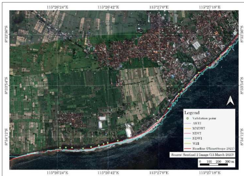
Figure 6-7. Result of coastline extraction using Normalized Difference Water Index (NDWI).
