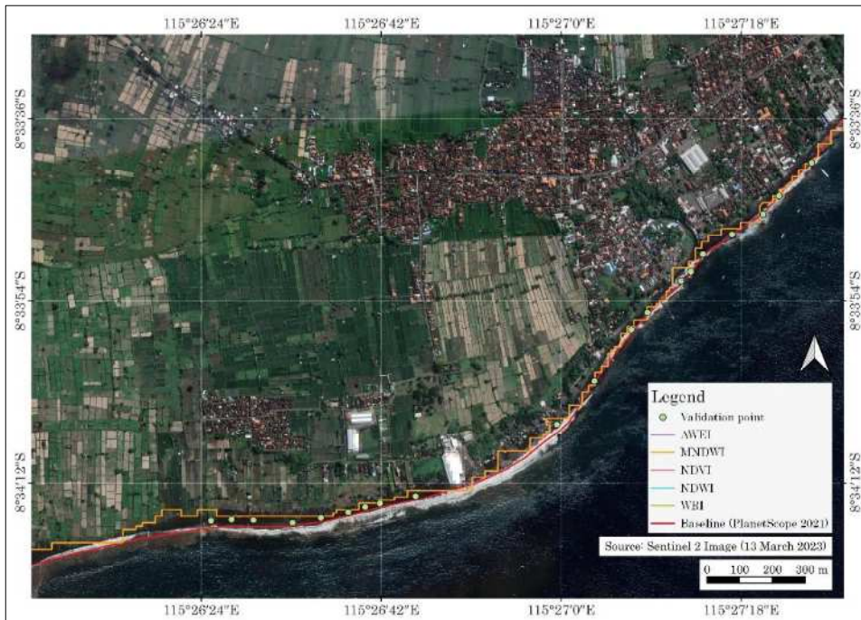
Figure 6-8. Result of coastline extraction using Modified Normalized Difference Water Index (MNDWI).
