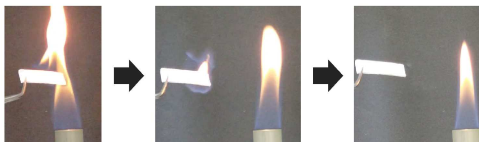
Figure A6.1 Flame test of the concentrated 3.2 \text{ mol dm}^{-3} LiFSA/TFEAc solution.
