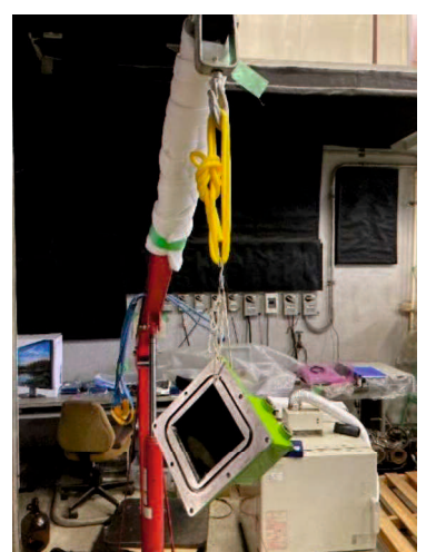
Fig. 2.8 Structural parts holding method (rubber tube with kite string)
