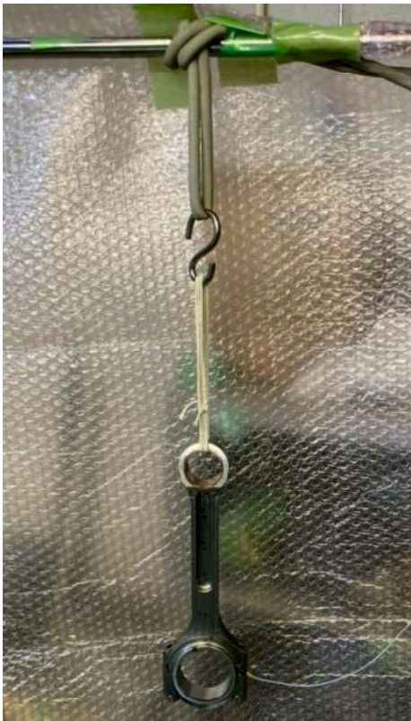
Fig. 2.10 Main motion system parts holding method (rubber tube with kite string)
