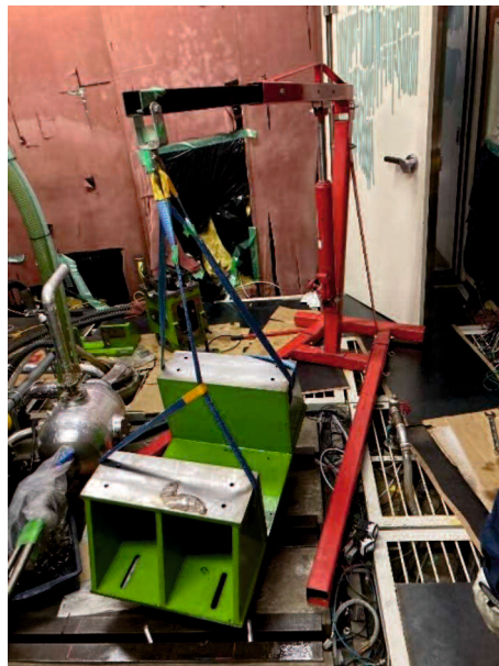
Fig. 2.16 Mount parts holding method (sling belt)
