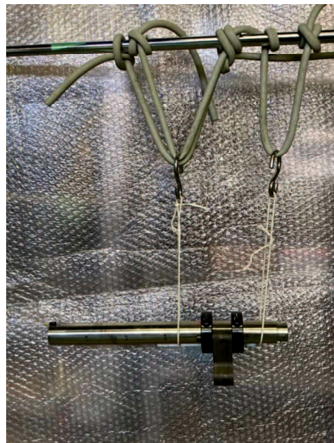
Fig. 2.10 Main motion system parts holding method (rubber tube with kite string)
