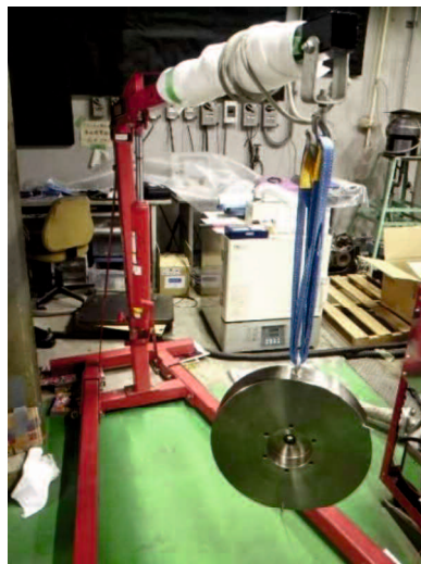
Fig. 2.12 Main motion system parts holding method (sling belt)
