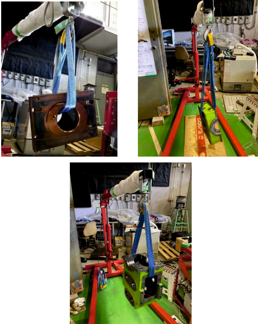
Fig. 2.9 Structural parts holding method (sling belt)
