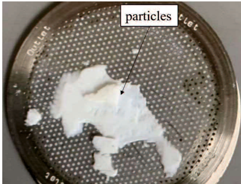
Fig. 2-20 photograph of particles formed during chemical vapor deposition on the membrane filter
