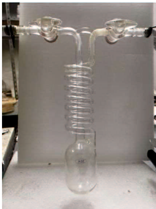
Fig. 2-3 Setting part of the trap
