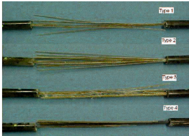
(a) GFRP rod failure [81]
