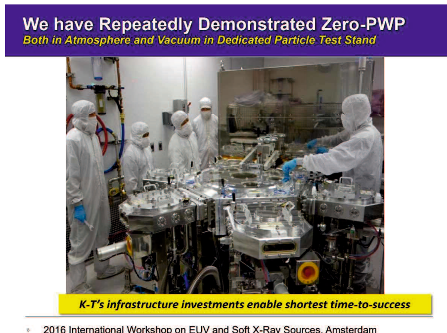
図 5-8 開発したアルミニウム合金製真空装置の写真 (出典 : 2016 International Workshop on EUV and Soft X-Ray Sources, Amsterdam, https://euvlitho.com/source-workshop/2016-international-workshop-on-euv-and-soft-x-ray-sources/ , (2022.02.09 取得)).
