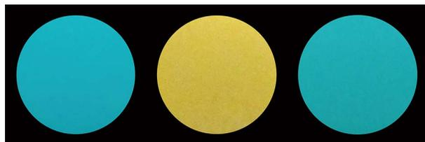
**Figure 10.** Fluorescence colors of a SSA–DPDP hybrid film in the as-prepared state (left), swollen state (middle), and dried state (right).
