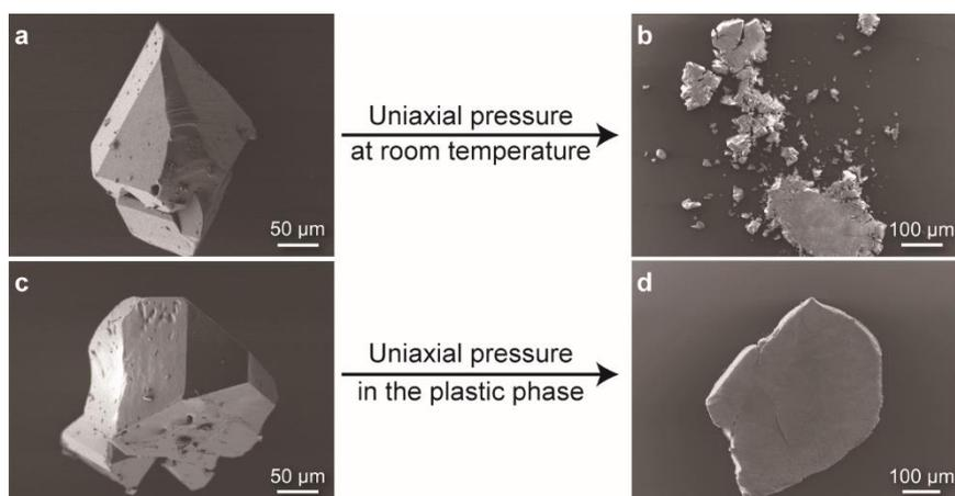
**Figure 5 | Phase-dependent pressure-induced morphology changes of crystals of 1.** **a** and **b**, SEM images of a single crystal of **1** before and after application of uniaxial pressure at room temperature (LTP). **c** and **d**, SEM images of a single crystal of **1** before and after application of uniaxial pressure at high temperature (HTP; plastic crystal phase).
