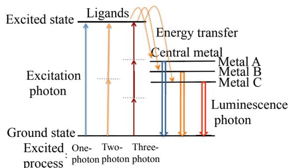
Figure 1. Schematic representation of one-, two- and three-photon induced luminescence from rare earth metal complex.
