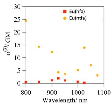
Figure 4. Three-photon absorption cross-section of Eu(ntfa) and Eu(hfa) at respective wavelength of excitation light source.
