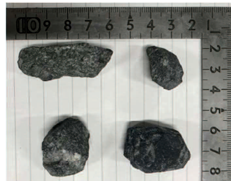
Fig. 4.14 Coarse aggregates with different sizes and shapes
