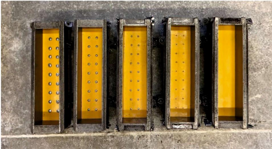
**Figure 5-1** Steel forms with wood plates having round screws
