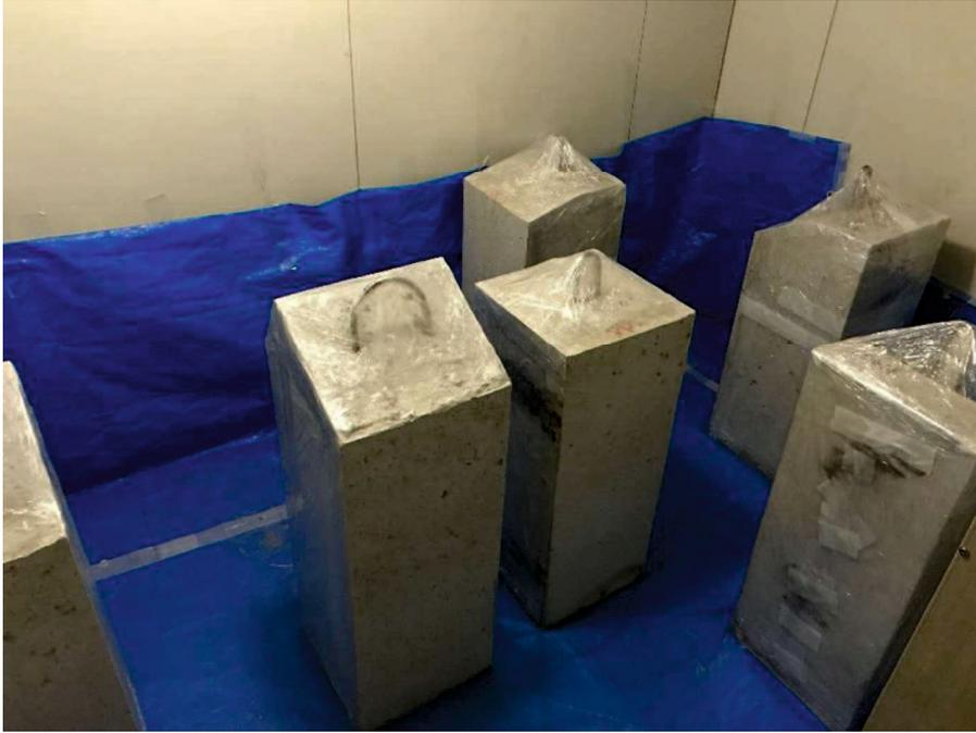
Figure 4-2 Specimens in the freezing chamber
