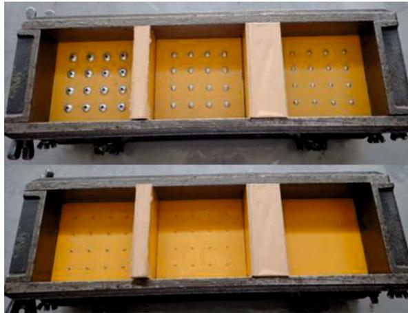
**Figure 3-1** Steel mold with wood plates having various sizes of round screws
