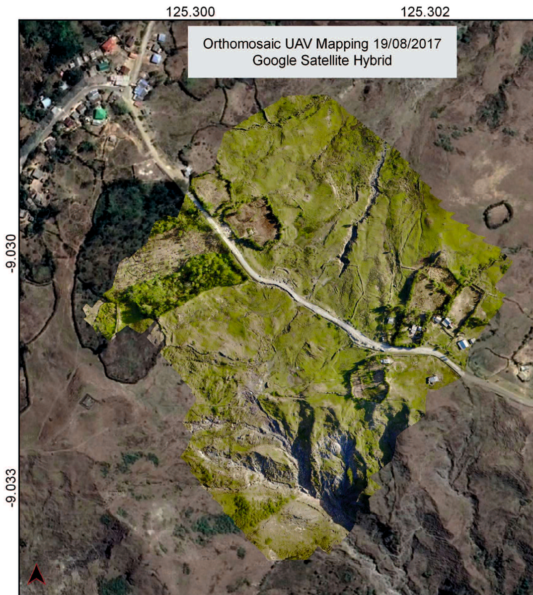
Figure 5.7. Unmanned Aerial Vehicle (UAV) orthomosaic image overlaid on Google Maps Hybrid
