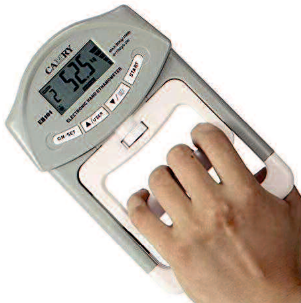
Figure 1.13 Digital Hand Dynamometer Grip Strength Measurement Meter used for measuring hand grip strength.
