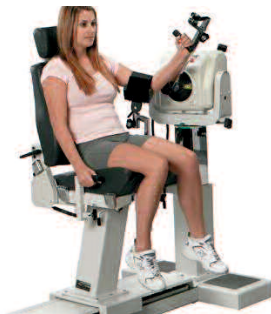
Figure 1.14 Dynamometers for assessing elbow flexor strength of the athletes. The Biodex System 4 [49].
