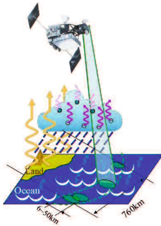
Figure 1.2. Sketch of rainfall measurement by PMW instrument, illustrated for the TRMM Microwave Imager (TMI) instrument aboard the TRMM satellite (Shimizu, 2009).
