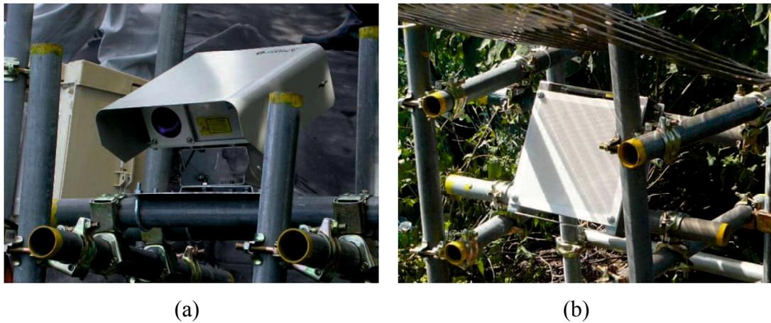
**Fig. 3.19.** Diffusion Laser Displacement Meter (DLDM, see Fig. 3.4): (a) DLDM and (b) Reflector.
