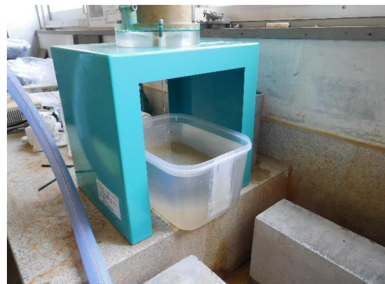
Fig-6 Schematic diagram of drainage and catching case
