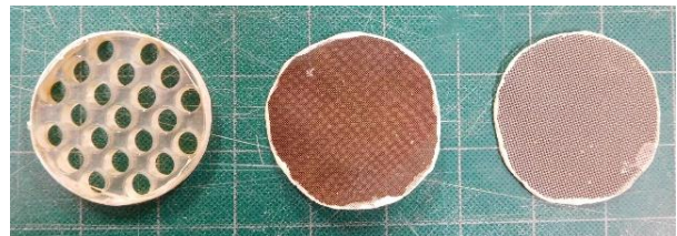
Pic-3 Acrylic plate and mesh (Acrylic plate, 250μm mesh, 425μm mesh)
