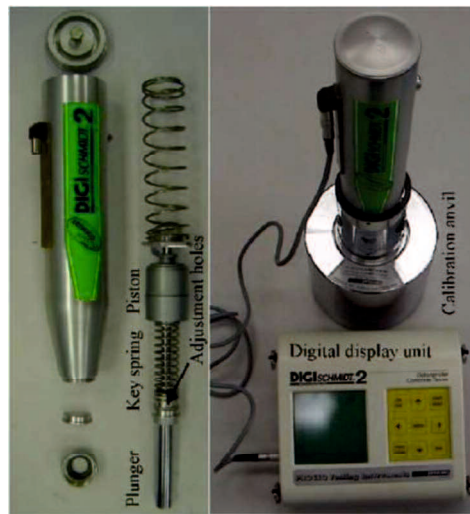
Fig.2.1 Components of Schmidt hammers 8) .
