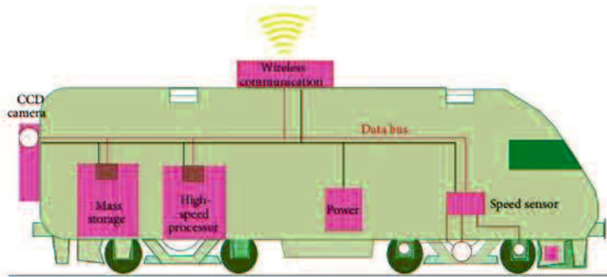
Fig.2.6 Diagram of development of VWMS on a train 21) .
