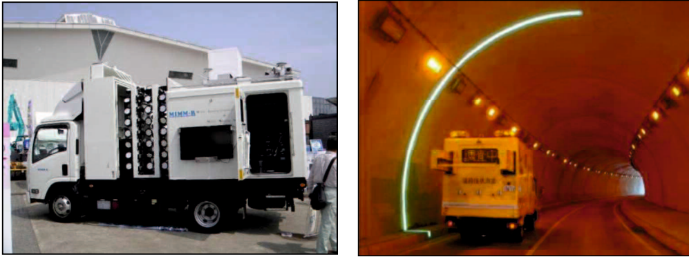
Fig.1.1 Image acquisition system using MIMM-R 6) .
