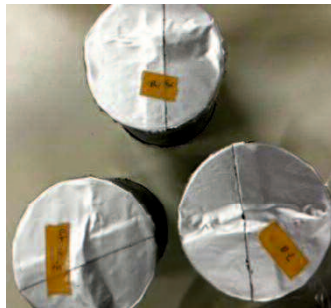
Fig. 3.2 Specimen's section sealed with waterproof tape
