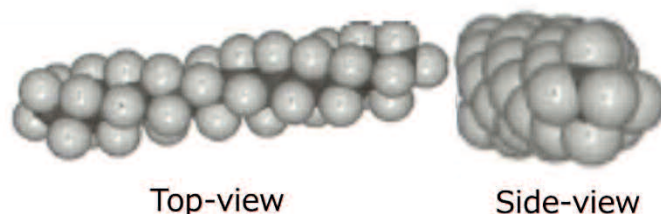
Figure 1-2. Molecular structure of perfluoroalkyl chain.
