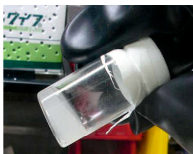
Figure 4-4. Gel electrolyte used in this chapter (1M- \text{LiPF}_6 , EC/EMC =1/2).
