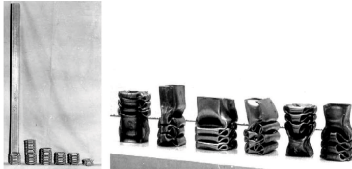
Figure 1.13. Axial deformations on rectangular tube [19].
