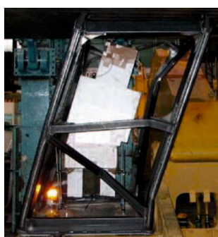
(a). Real experiment testing of cab frame (conventional method).
