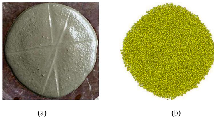
Fig. 4.5 The final shape of the series No. 1 fresh mortar on the flow table: (a) experiment (mean flow value: 210 mm), and (b) numerical simulation (mean flow value: 212 mm )
