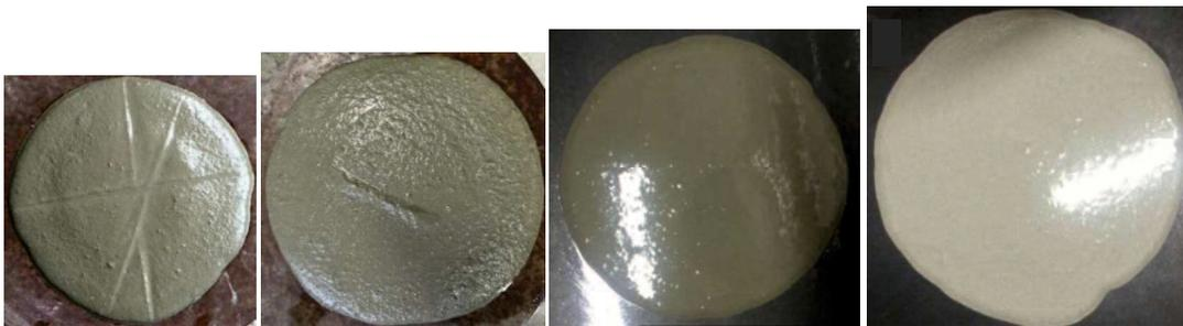
Fig. 3.4 The final shape of the series No. 1-4 fresh mortar on the flow table
