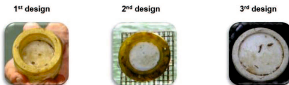
Fig. 2.4 Different housing designs of Chemcatcher® device. (Source; Charriau et al., 2015)
