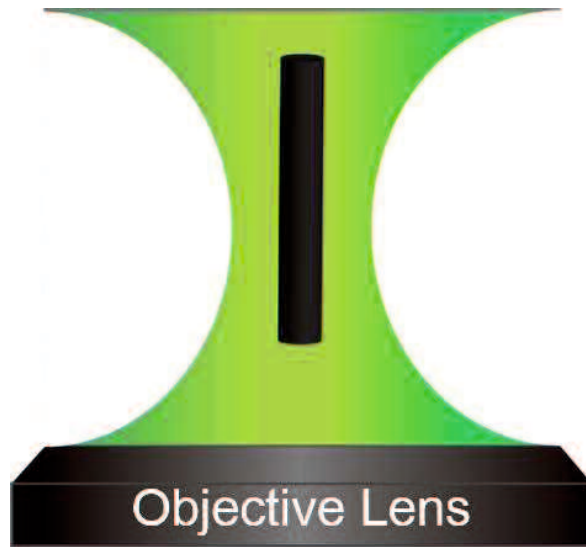
Figure 1-6. Schematic representation of an optically trapped one-dimensional rod-like material by a tightly focused laser beam.
