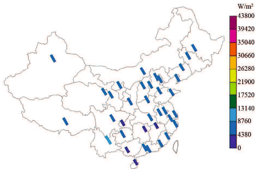
(b) Natural ventilation potentials of 36 selected cities; the highest value in the label represents the annual sum of the internal gains
