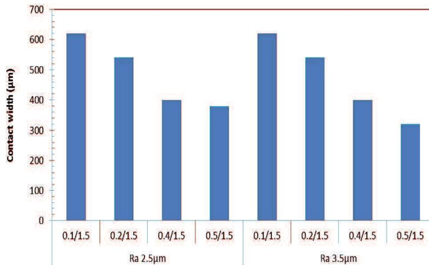
Figure 5.37 Contact width simulation result for all level real surface roughness model of flange and all thickness ratio when axial force 120kN [400MPa mode]
