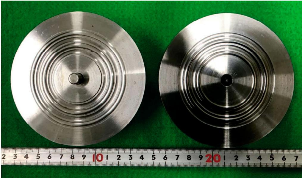
Fig.5.1 The upper and lower dies
