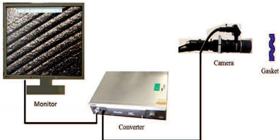
Fig. 5.35 Digital microscope VH-Z250
