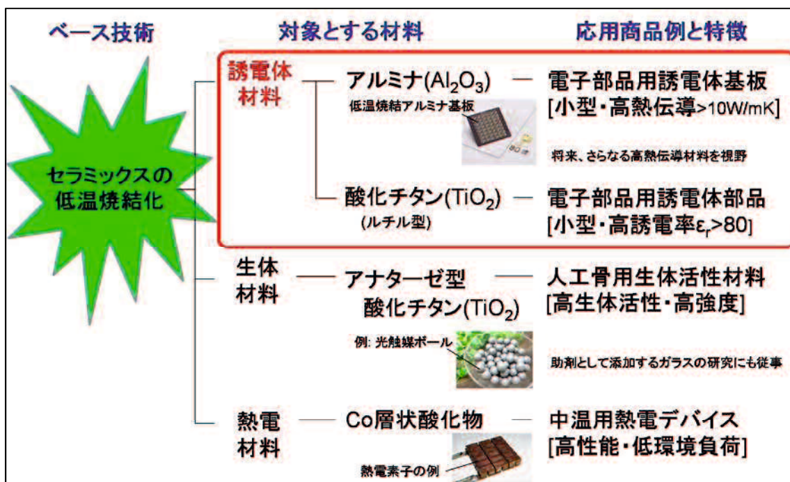
Fig. 1.1 Bird's eye view of aimed materials, examples of application and features based on low-temperature sintering technology of ceramics.
