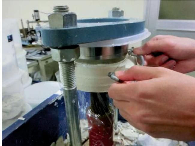
Figure 3. 12 A soil specimen in process of trimming
