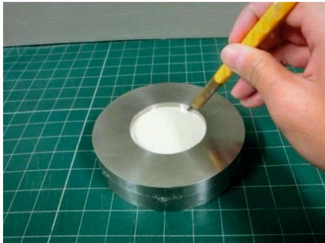
Figure 3. 13 Removing the inside soil core to make an annular specimen
