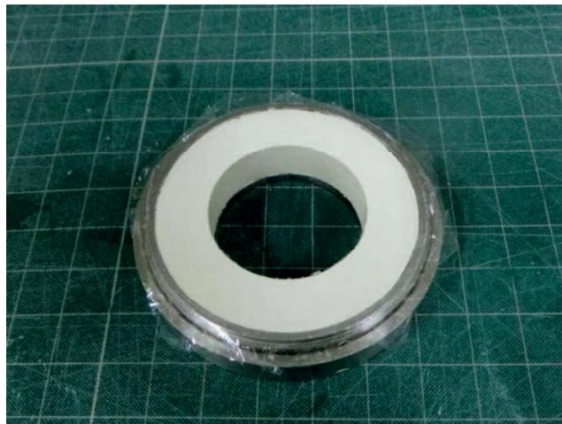
Figure 3. 14 Completing specimen before transferring to the shear box
