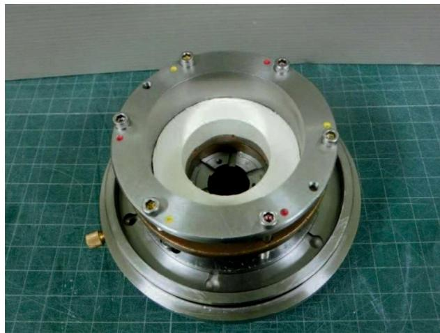
Figure 3. 16 Final setting before ring shear test
