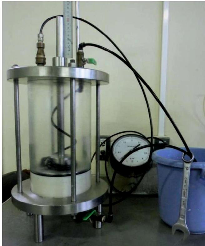
Figure 3. 11 Soil specimen in process of pre-consolidation
