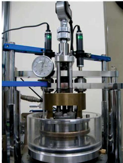
Figure 3. 7 Shear box containing test sample
