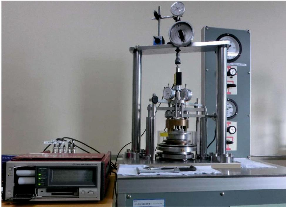
Figure 3.2 Front view of ring shear-test apparatus
