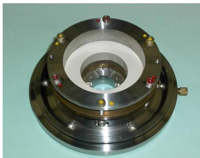
Photo.2 Annular specimen in ring shear box
