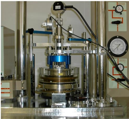
Photo.1 Ring shear test apparatus
