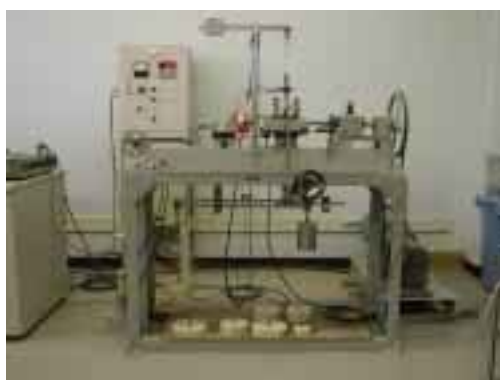
Photo. 2 Reversal box shear test apparatus (After Nakamori et al. 1996)
