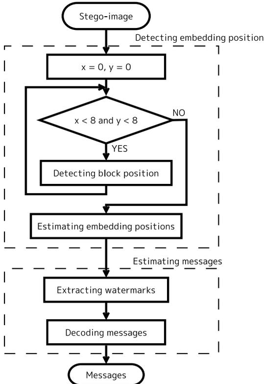
Fig. 4 Decoding process.
