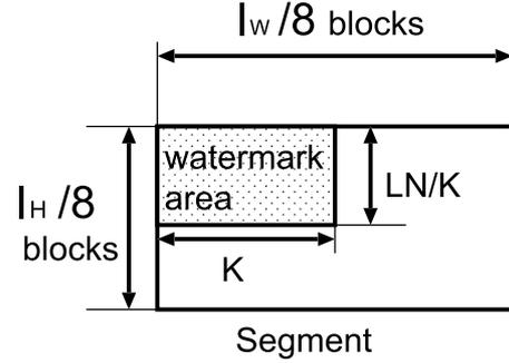
**Fig. 3** Watermark area in a segment. Size of watermarks is  $\lceil \frac{LN}{K} \rceil \times K$  blocks.
