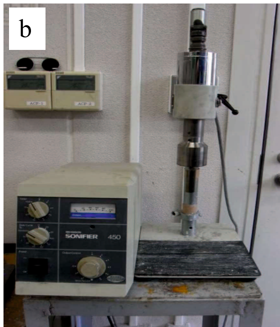
Fig. 2.4 Overview of (a) mechanical stirring device and (b) ultrasonic homogenizer.
