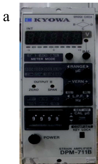
Fig. 2.9 Overview of (a) strain amplifier and (b) strain gauge.
