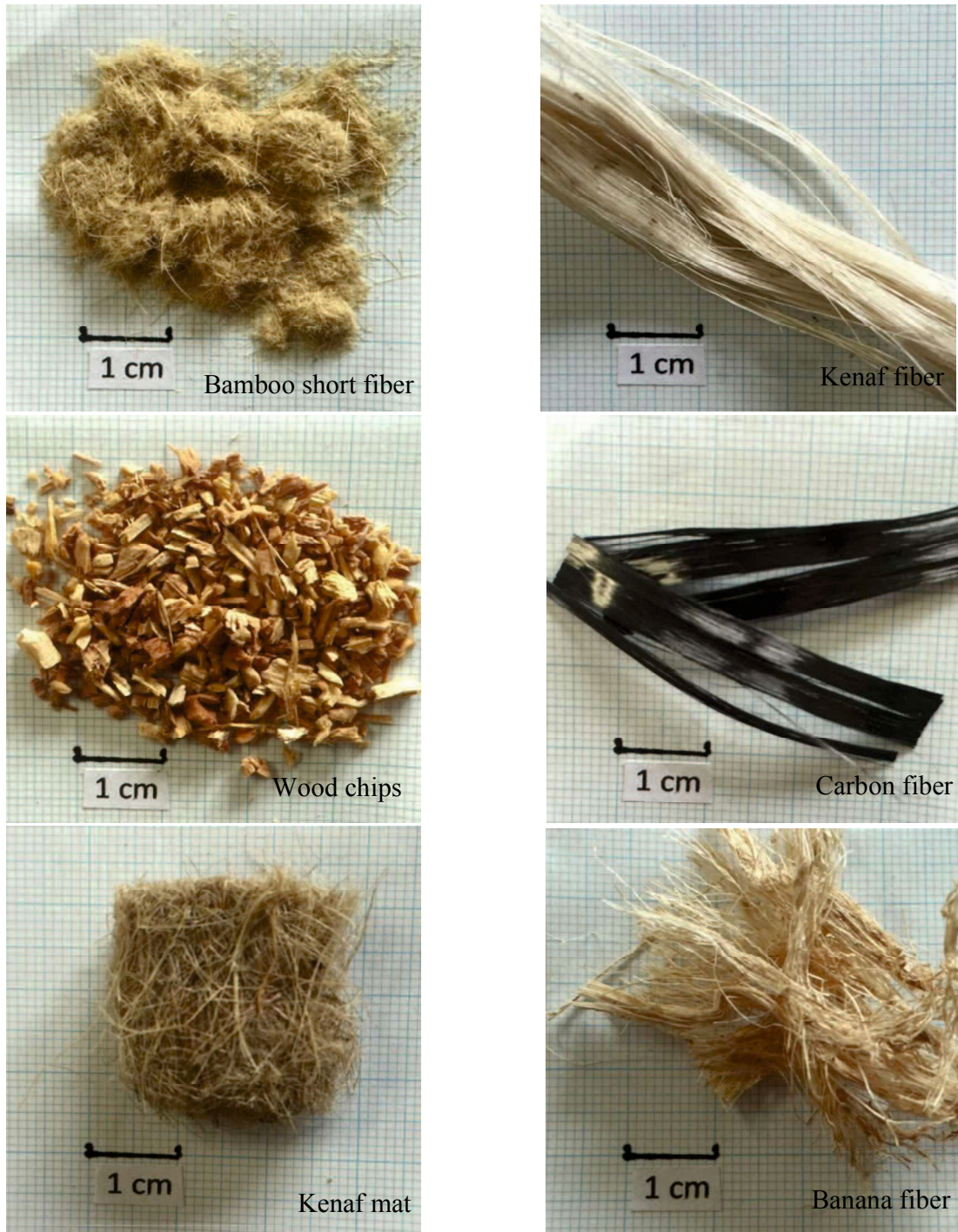
Fig. 1.2 Different types of reinforcements applicable to fabricate composite materials.
