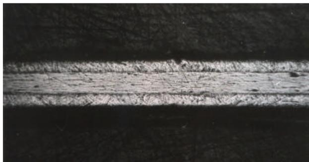
Fig.1 Optical micrograph of longitudinal cross-section of Nb<sub>3</sub>Al tape.
