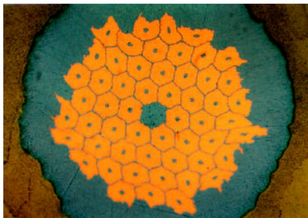
Fig.2 Optical micrograph of cross-section in Jelly-rolled Nb<sub>3</sub>Al wire after ohmic-heating.
