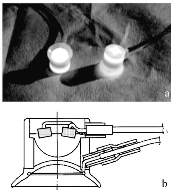
Fig. 1. Contact electrode with built-in diode light source. (a) Photograph of LED-electrode (flashing). (b) Schema of LED-electrode in section. Three or four light-emitting diodes are built into the contact electrode.
