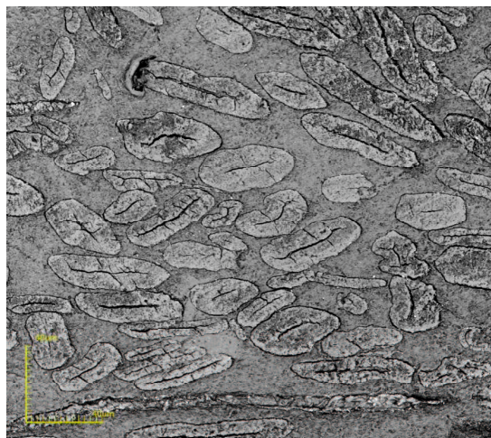
Figure 2.14 Laser micrograph of transverse section of short ramie/PP reinforced composites produced at 195°C during Process B.
