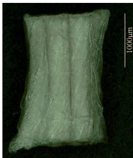
Figure 2.6 A chopped pellet containing six ramie single yarns by M-PaRI included process.
