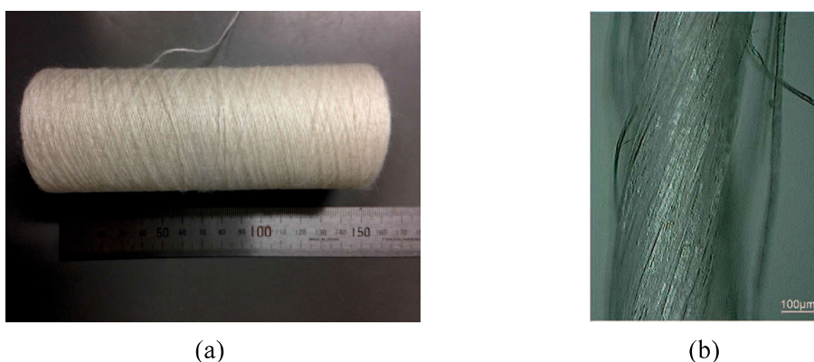
Figure 2.1(a) Aspect of ramie spun yarn on a textile bobbin. (b) Magnified observation of a ramie spun yarn
