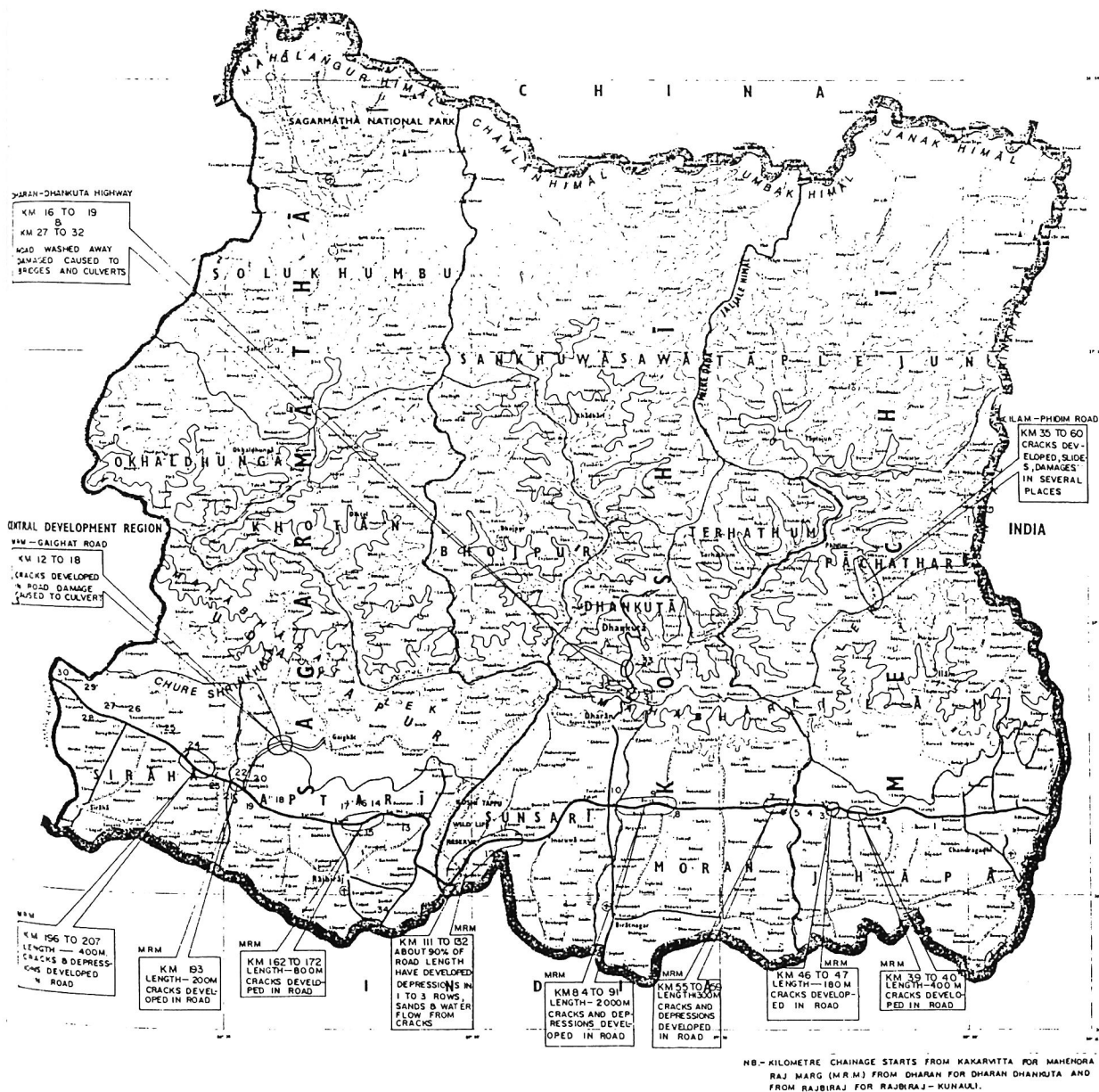
Fig. 3.7 Damage to roads in the eastern development region of Nepal
