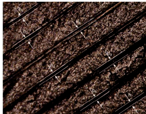
(d) surface roughness of gasket after contact with flange having surface roughness 3.5\mu\text{m}
