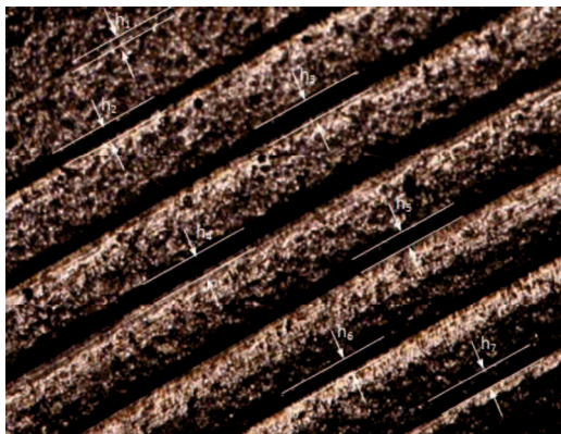
(c) surface roughness of gasket after contact with flange having surface roughness 2.5\mu\text{m}
