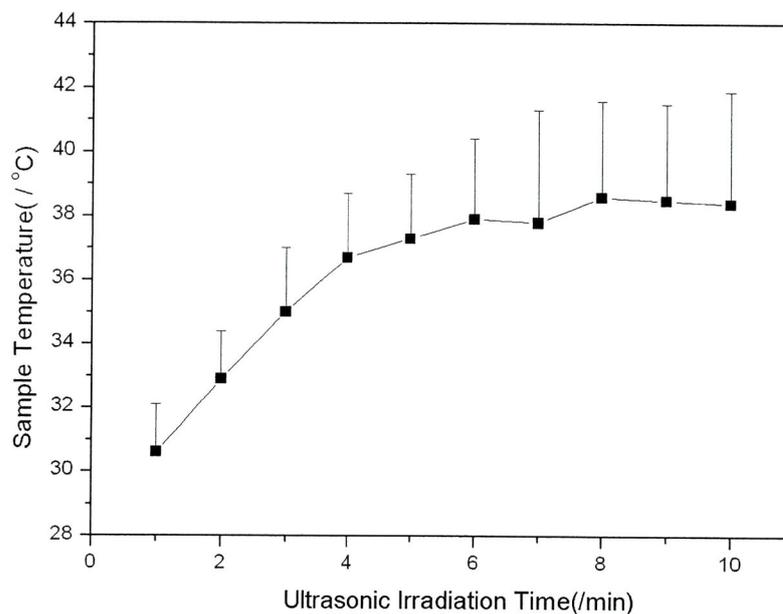
Fig. 3.4 Relationship of sample temperature and ultrasonic irradiation time
