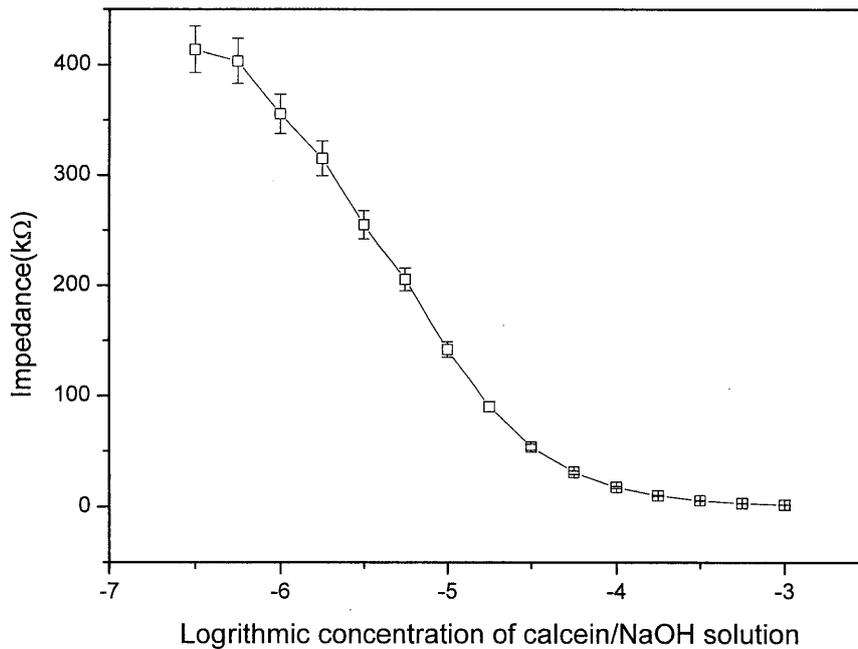
Fig. 5.3 Relationship between impedance (real part) and Calcein/NaOH solution concentration.
