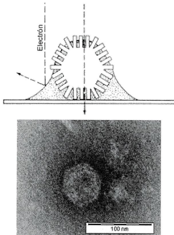
Fig. 2.12 Schematic representation of a specimen particle (e.g., liposome) in TEM observation.
