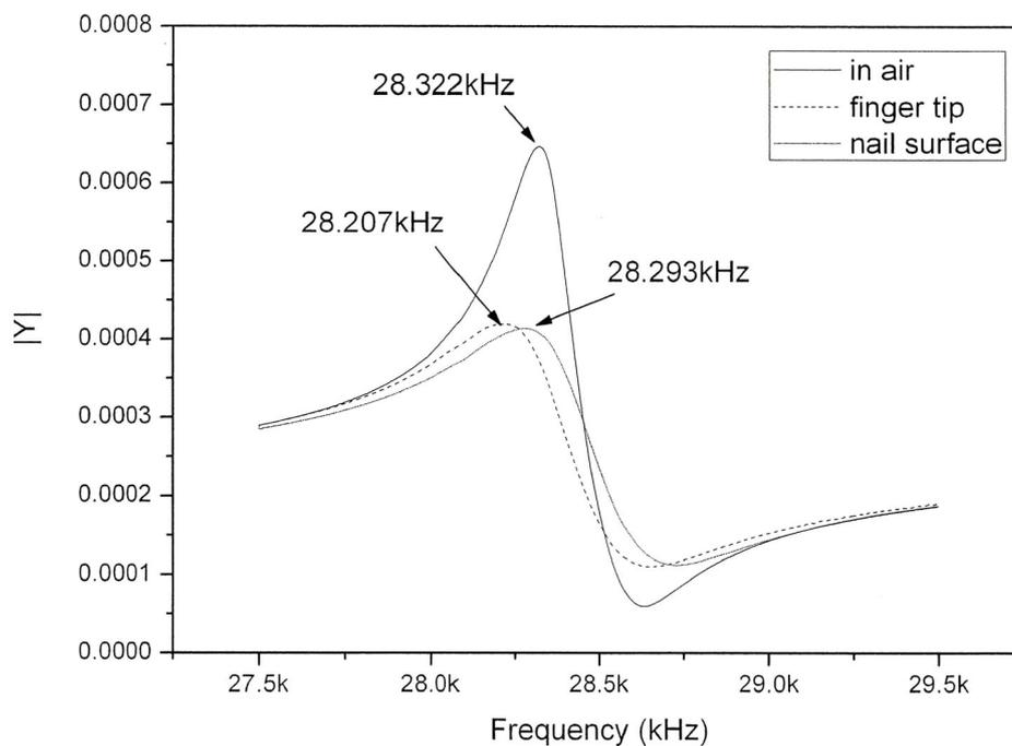
Fig. 4.5 Admittance frequency responses obtained when the ultrasonic probe attached to different objects.
