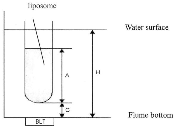
Fig. 3.15 Dimension of the sample in the water flume where  $A = 28\text{mm}$ ,  $H = 50\text{mm}$ ,  $C = 1\text{mm}$ .
