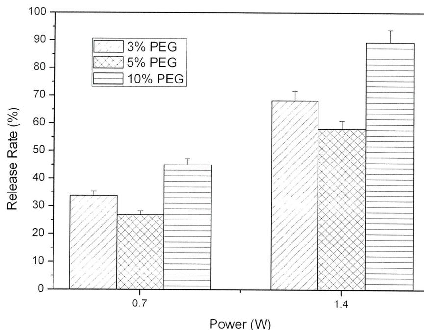
Fig. 4.6. Average release rates of each sample after 120 seconds irradiation at 28.18 kHz with adjusting the input power. Mean S.D. n=4
