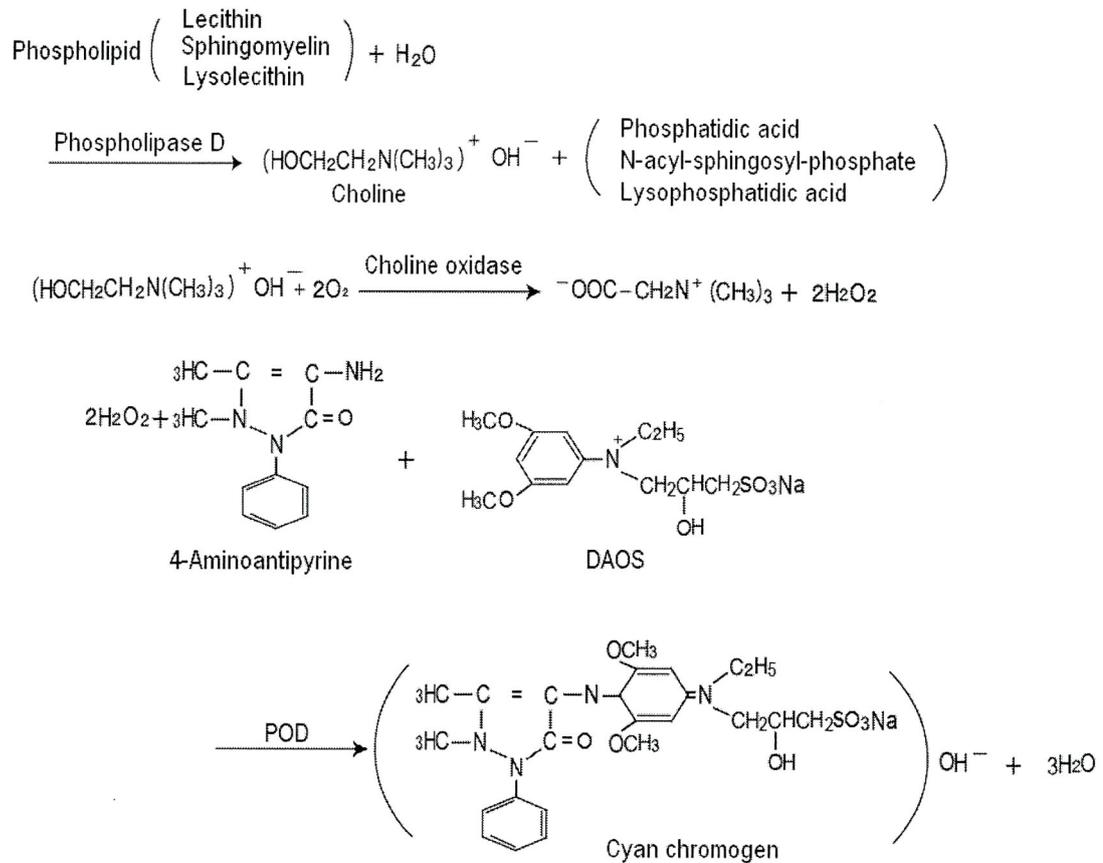
Fig.2.8 Chemical reaction equation of DOAS method
