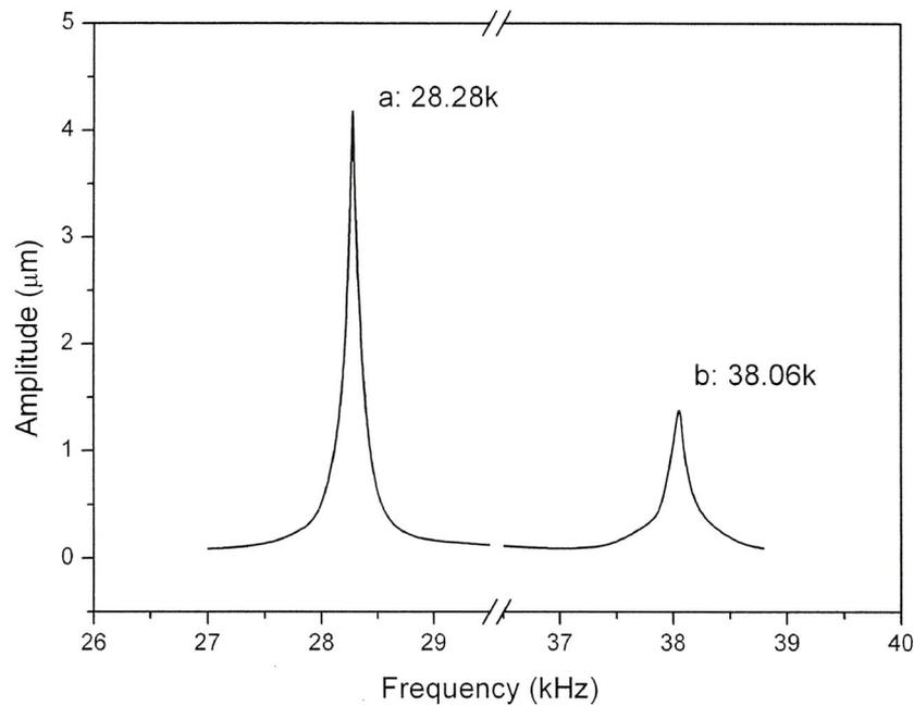
Fig.4.2. Frequency response of the tip displacement of probe at a constant input voltage 10Vp-p.
