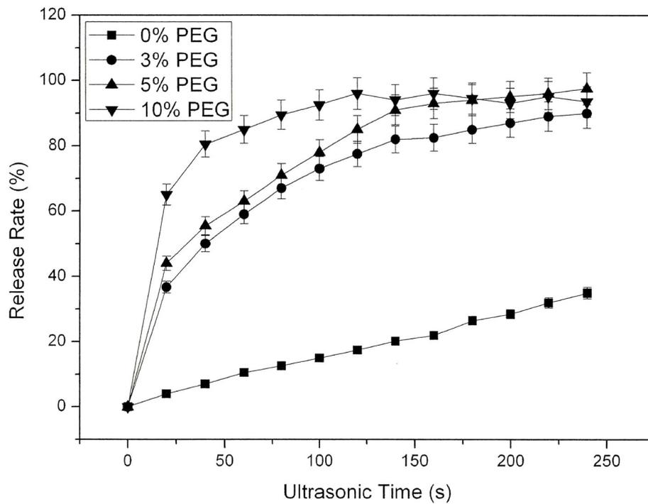
Fig. 3.16 Release rates of calcein liposomes of different PEG amount induced by 45kHz ultrasound with an ultrasound cleaner. Mean  $\pm$  S.D.  $n=4$ .
