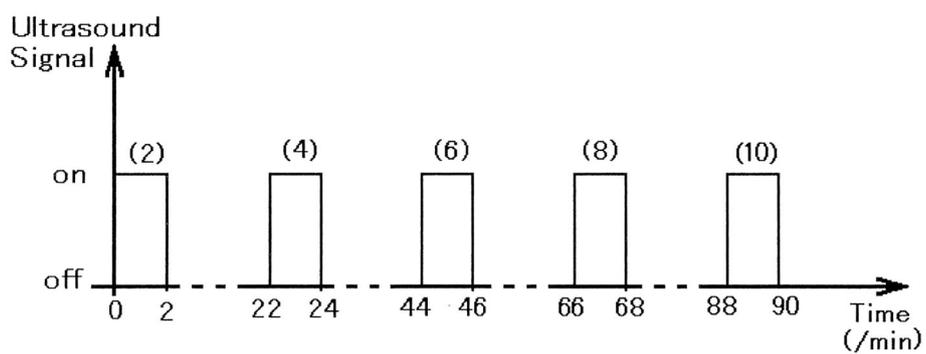
Fig.3.3 Pulsed power mode of ultrasonic irradiation
