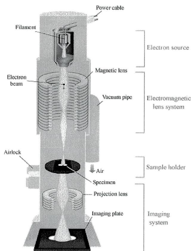
Fig. 2.10 Schematic structure of a TEM
