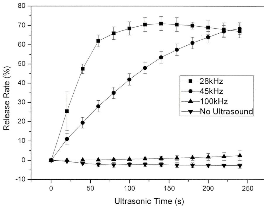
Fig. 3.14 Release rates of calcein liposomes induced by different frequencies ultrasound with an ultrasound cleaner compared by that without ultrasound treated sample. Mean  $\pm$  S.D.  $n = 4$ .
