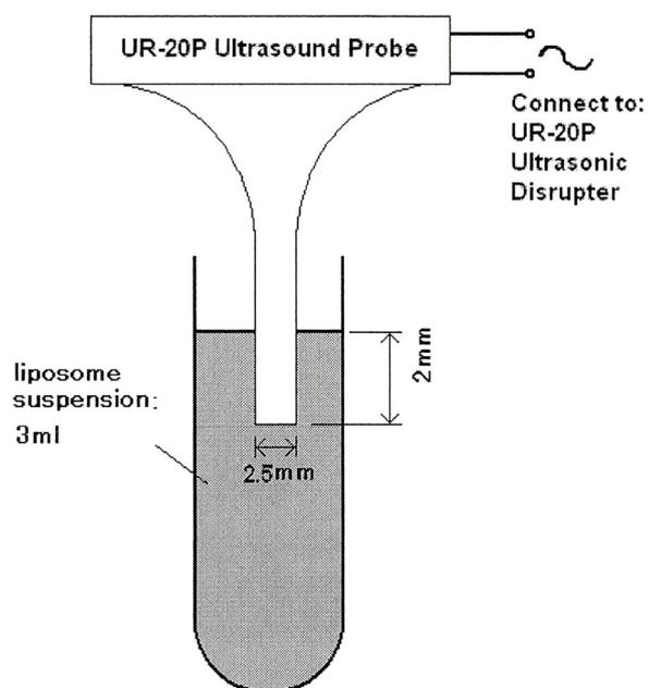
Fig. 3.2 Schematic diagram of ultrasonic irradiation
