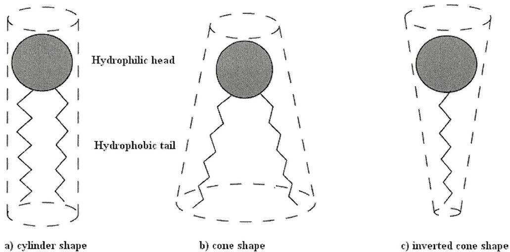
Fig. 2.1 Three basic molecular shapes of amphiphile: a cone, a cylinder, an inverted cone.
