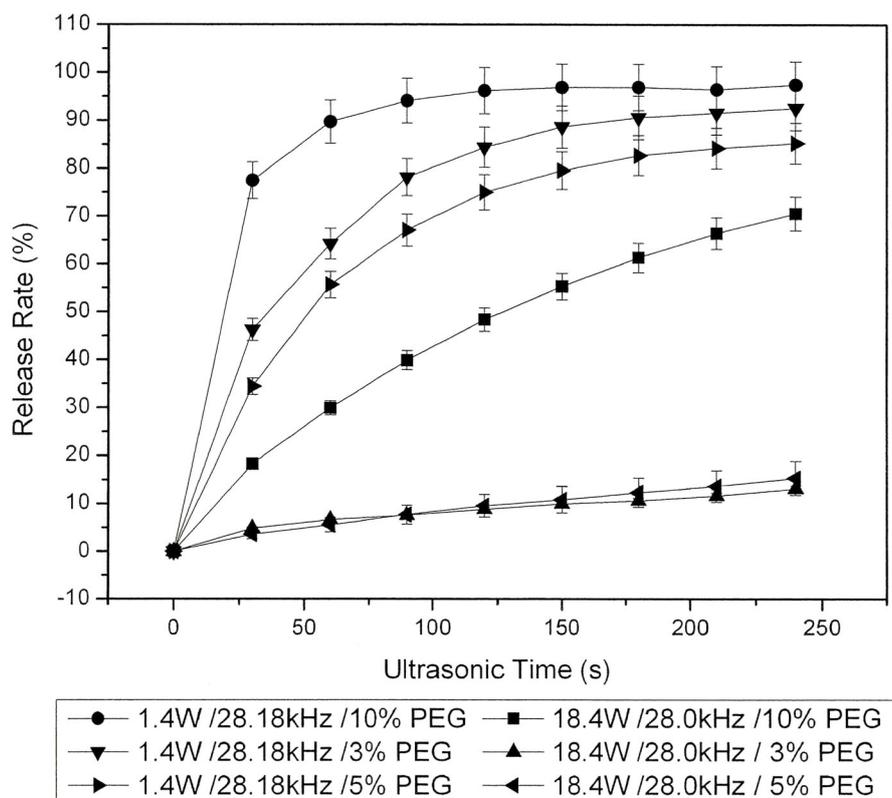
Fig. 4.7. Release effect comparison of the input at 28 kHz with 18.4W to 28.18 kHz with 1.4W.
