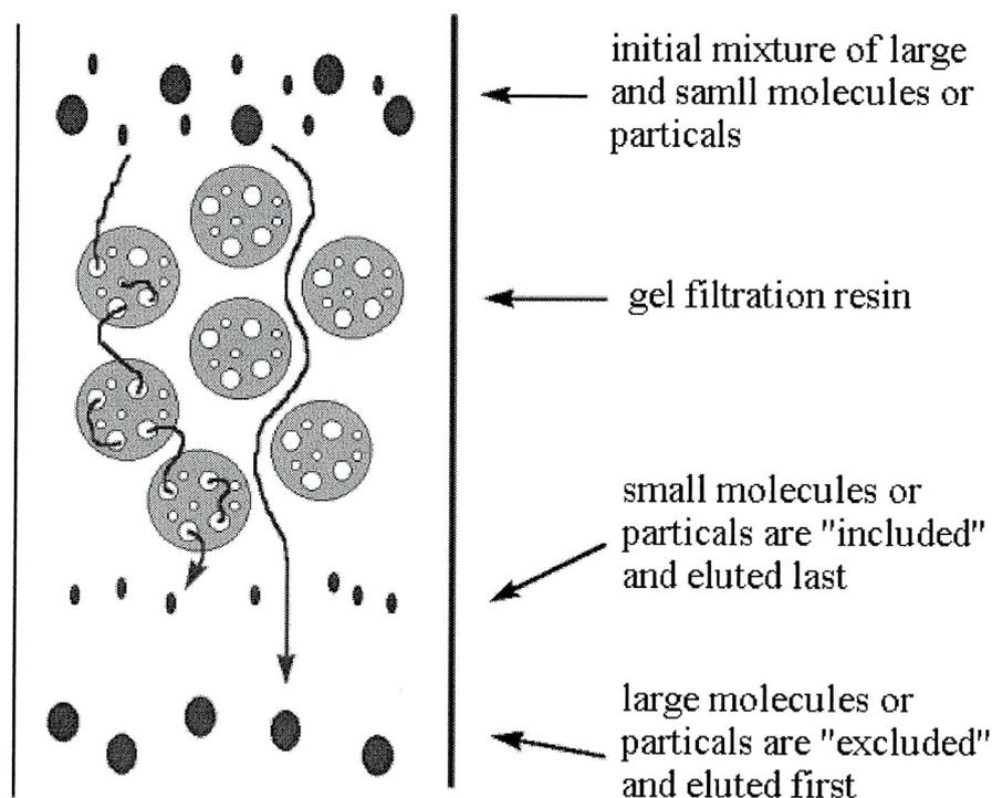
Fig. 2.7 Schematic of gel filtration
