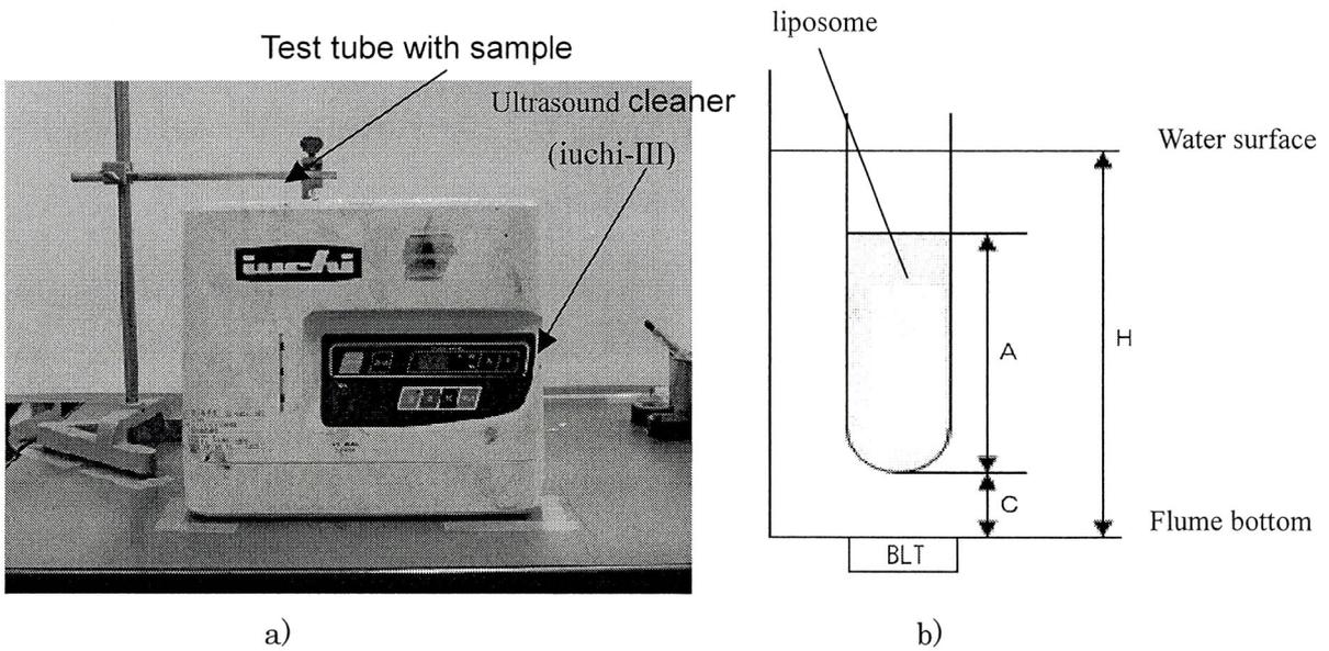
Fig. 3.13 Ultrasound induced release experiment setup and the dimension of the sample in the water flume where  $A = 35\text{mm}$ ,  $H = 60\text{mm}$ ,  $C = 1\text{mm}$ .
