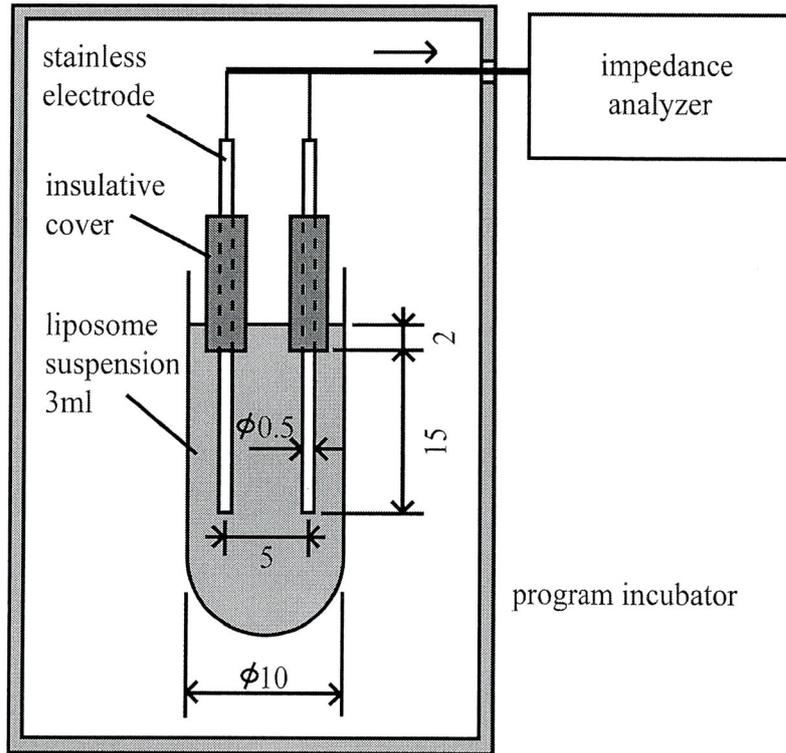
Fig. 5.2 Impedance measurement system setup
