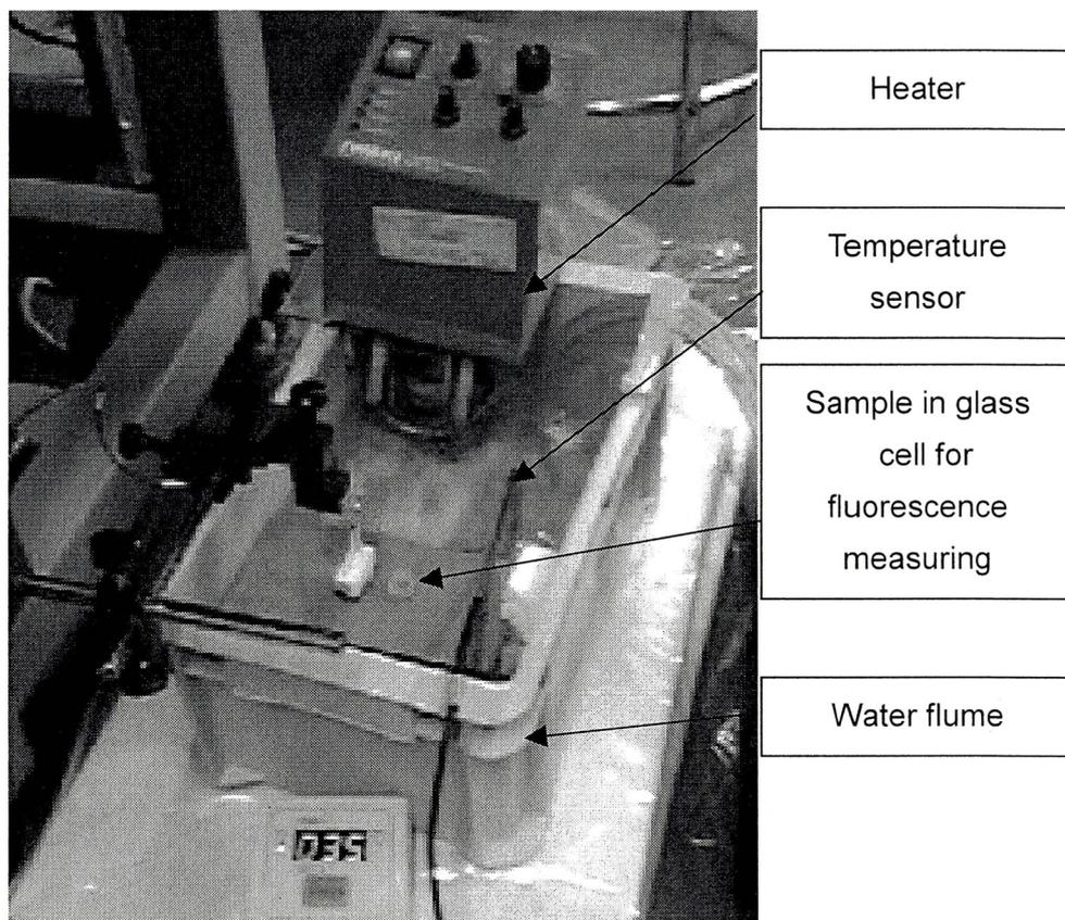
Fig. 3.11 Temperature induced release experiment setup
