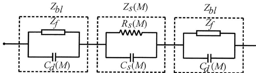
Fig. 5.1 Equivalent electrical model of solution impedance measurement
