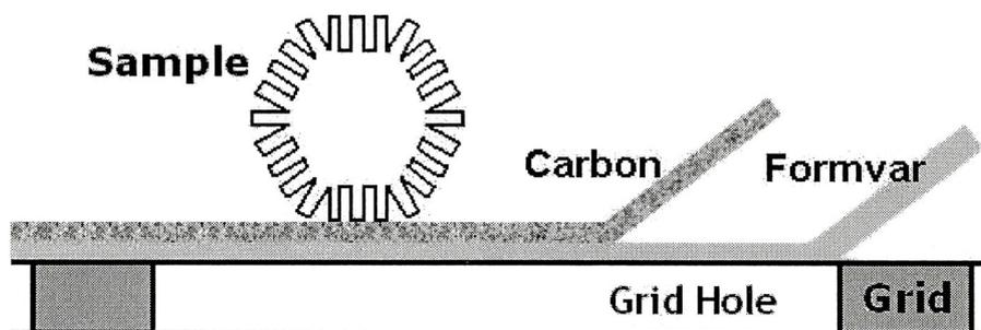
Fig. 2.11 Schematic of liposome specimen for TEM
