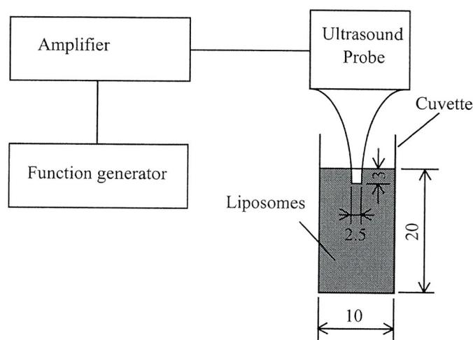
Fig.4.1. Ultrasonic irradiation experiment setup.
