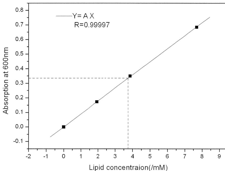
Fig. 2.9 Relationship between lipid concentration and absorption at 600nm.
