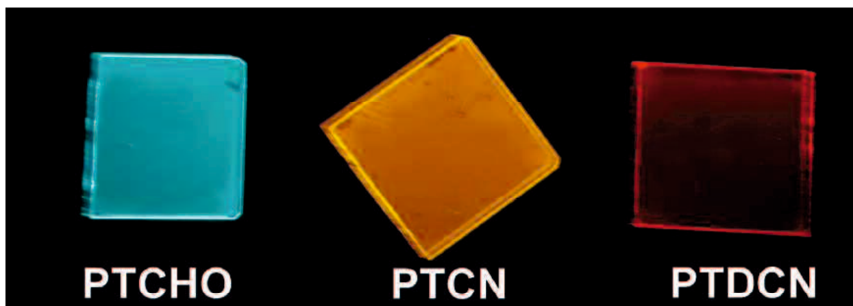
Figure 2-1 Fluorescence of the spun films of PTCHO, PTCN, and PTDCN under UV irradiation ( \lambda_{\text{ex}} = 365 \text{ nm} ).
