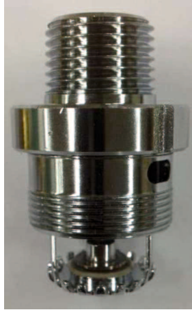
Figure 3.7 K-50 sprinkler test specimen
