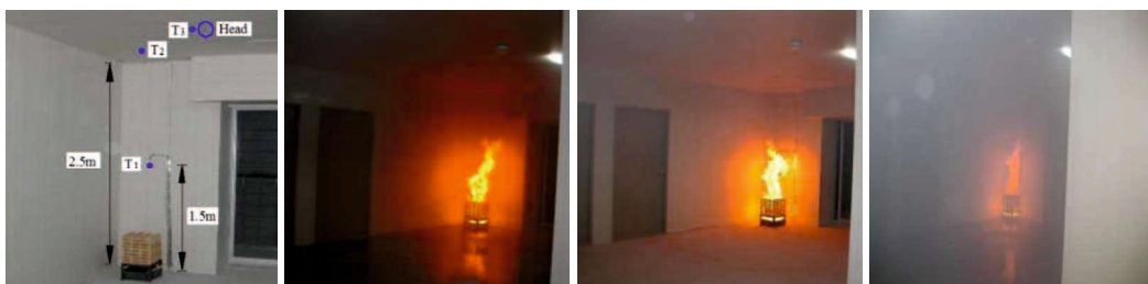
Figure 5.6 Fire ignition and suppression sequence during the actual fire test
