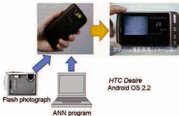
Figure 1. Dust measuring system using mobile phone camera.
